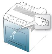
2. Carefully remove the paper by pulling in the direction as shown below.
